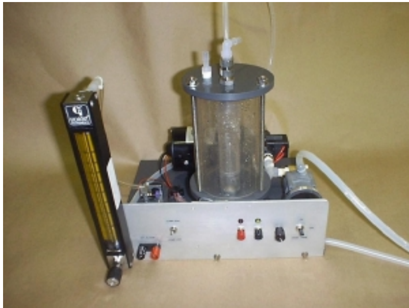
Figure 7. Equilibrator and control system in SeaKeepers submodule
