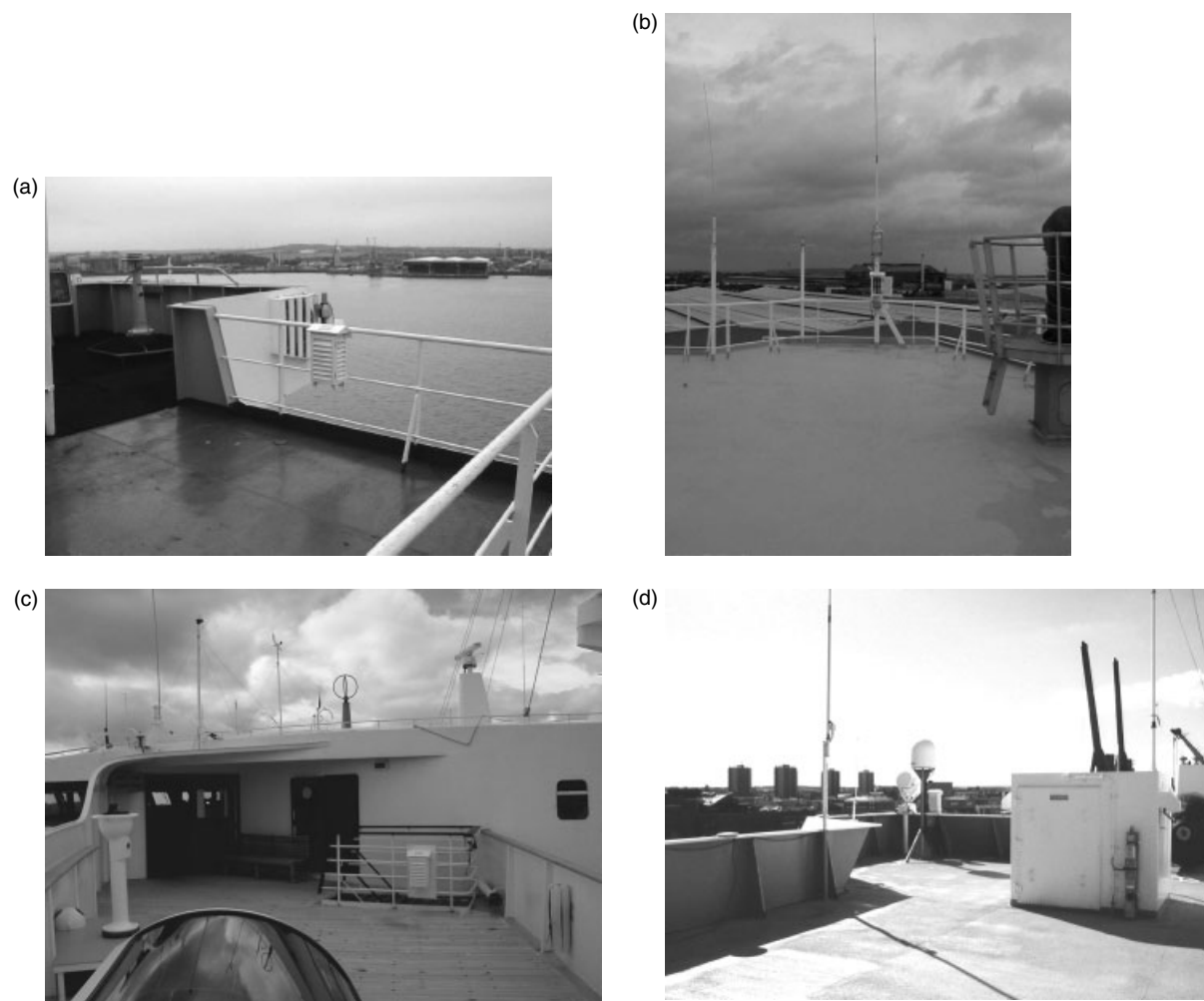
Figure 1. (a) Starboard screen on board the City of Cape Town (GXUP). The screen has been categorized as having a medium exposure, due to being mounted on open railings, low down and back from the leading edge of the bridge wing. (b) Port screen on board the Dominica (C6LF9). The screen has been categorized as well exposed, due to being mounted in an exposed location on the wheel-house top, against open railings and mounted relatively high above the deck. (c) Port screen on board the Queen Elizabeth II (GBTT). This screen has been categorized as poorly exposed, due to being close to the deck in a relatively sheltered location and against a solid board. (d) Starboard screen on board the James Clark Ross (ZDLP). The screen has been poorly exposed, since it is low down, slightly above a solid metal railing. The screen is also far back from the leading edge of the wheel-house top and situated next to a spotlight
