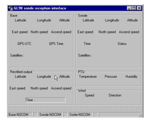
A special departure procedure shows the status of all parameters in the radiosonde transmitter insuring a safe launching of the balloon :
