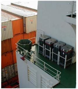
The balloons are filled with helium drawn by pipe from helium cylinder racks and are then attached to the radio sonde which carries sensors for measuring temperature, humidity and pressure. Wind speed and direction is most commonly calculated with a GPS module (although Loran is also used in some cases).
