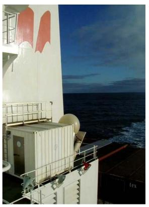
Balloon launching can be performed from transportable deck launching appliances or, alternatively, from a dedicated fixed 10 foot (3.05 metre) container.
