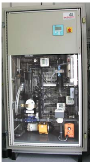
Fig. 4: Industrial version of a FerryBox (4H-Jena, Germany)
