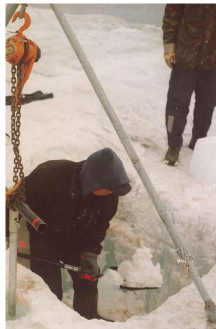
Figure 26 Pit dug attempting to retrieve corer
