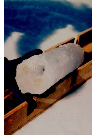
Figure 8 Drainage channel, algae in bottom core at Griffith site, 16 June (JD167)
