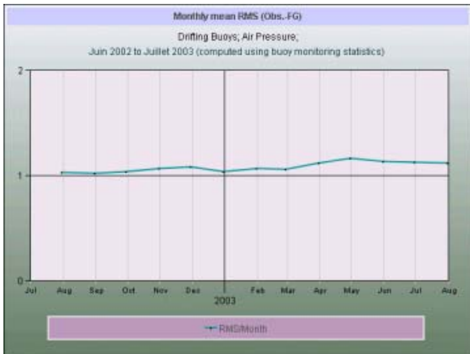
Graph 4: Evolution of mean RMS (Obs.-First guess) per month for the period June 2002 to July 2003 for global GTS air pressure data (from ECMWF monitoring statistics)
