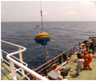
Fig1. Buoy system and BPR during deployment level
