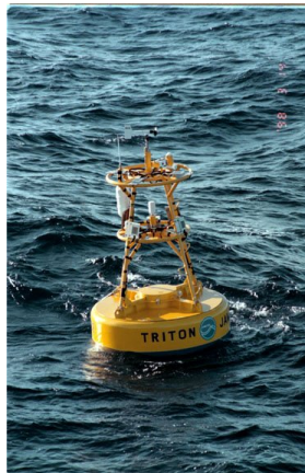
TRITON moored buoy (Western equatorial Pacific) http://www.jamstec.go.jp/jamstec/TRITON/
