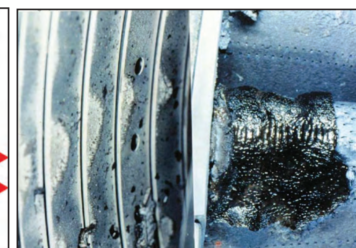
Ash deposits inside the jet engine that encountered the ash cloud from Redoubt Volcano 1989. Right: Dark glassy deposits of melted volcanic ash on leading edge of high-pressure turbine nozzle guide vanes. Left: Accumulation of unmelted volcanic ash in the high-pressure turbine rotor.
