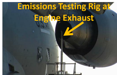
Sensor probes in emissions testing rig manifold
